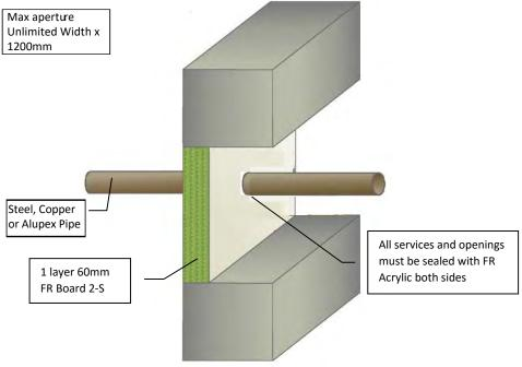
Smoke-Safe (<0.1m<sup>3</sup>/h smoke leakage at 200Pa)
